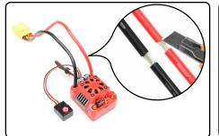
Using the cutter, carefully cut a piece of the ESC wire insulation to reveal the strands. Be careful not to cut the strands !
