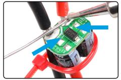
Check that the polarities are correct. Solder the capacitor to the ESC wires. Make sure that the weld is correct and durable.
