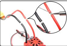
Using the soldering iron, preheat the strands for a few seconds and then apply the solder. Only the surface strands must be tinned.
