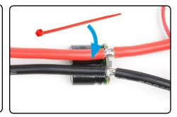
Place the capacitor on the ESC wires and hold in place with a tie-rap.
